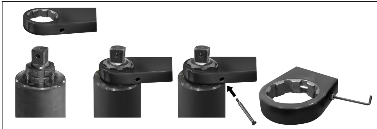
Figure 1: Socket Head Shoulder Bolt Install
