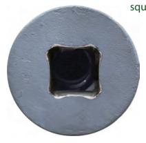
square-up a worn female socket with just a few hits of a hand-held, 4140-steel Swage Tool with our no rebound Dead-blow Hammer.
