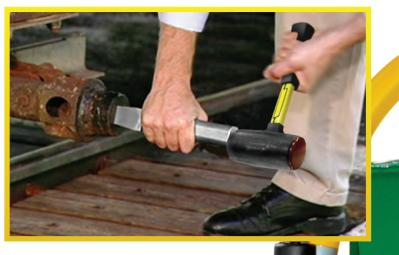
Fully Engage the Drive Fitting into the Capstan, AND OPEN THE GATE!
